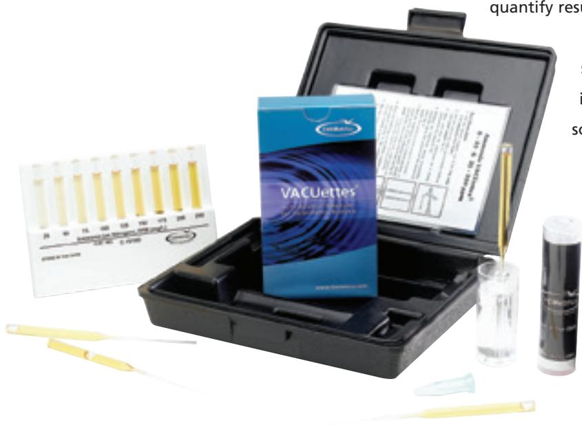
VACUettes ampoules are designed for highly concentrated samples. They employ a patented auto-dilution feature that eliminates the need for a time-consuming and error-prone preliminary dilution. As a result, the entire test typically takes only
